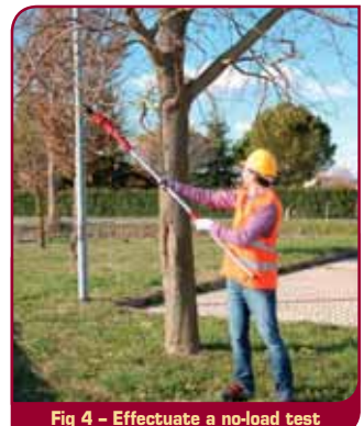
Fig 4 - Effectuate a no-load test
